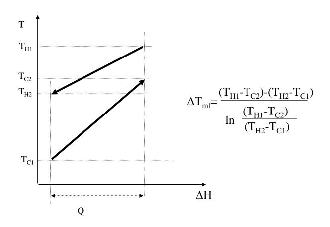
Since area= $Q/(U \Delta T_{ml})$ , the composite curve diagram provides one way of estimating the total area involved. Isolate all regions with a pair of straight line sections and calculate the area for each.
